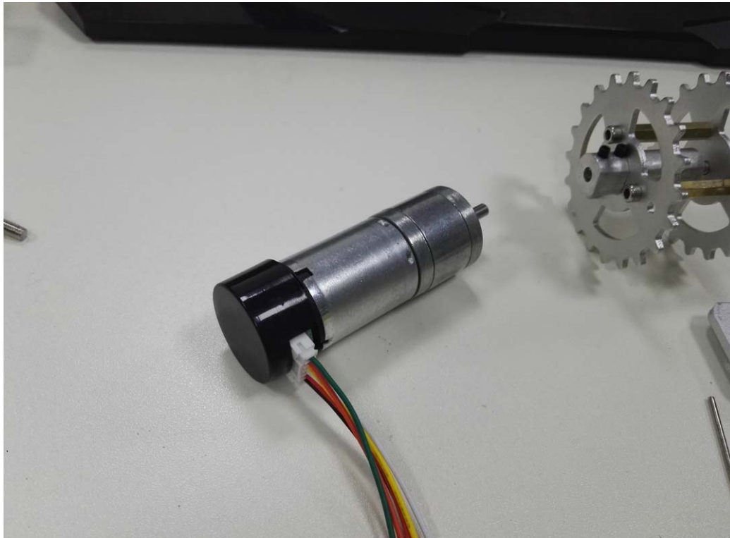
The motor cap is mounted on the motor, and plugged in motor line.
