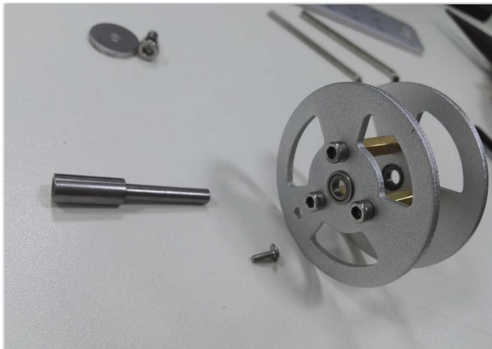
Place the bearing on both sides of the central round hole of bearing wheel
